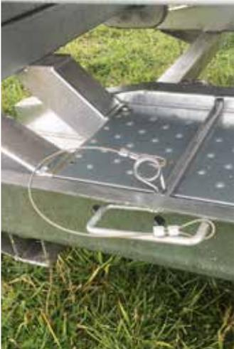
1. Remove, store and secure (with R-clips) the four locking pins restraining the skids of the feeder.
