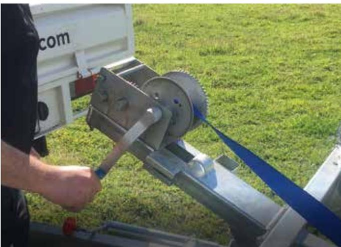
8. Fit the winch handle to the desired gear and winch the feeder up onto the deck.
