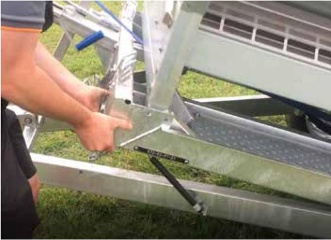
7. Take up any slack in the web strap using the winch handle. Store winch handle and re-engage winch clutch. Tilt feeder quickly to assist slide off.
