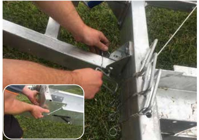
2. Remove and store pivot locking pin and tilt deck.
