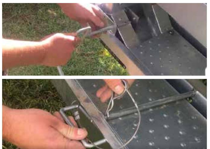
9. Apply locking pins to the four locations at the front and back of feeder and secure with R-clips.
