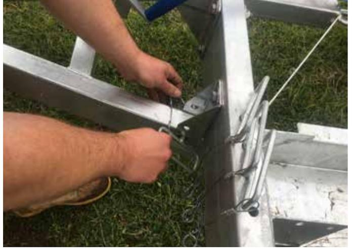
10. Apply pivot locking pin and secure with R-clip.
