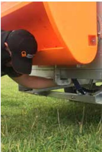
5. Remove the rear pull bar from the back of the feeder. Unhook the web strap from the pull bar. Attach hook to the eyelet at the back of the trailer.
