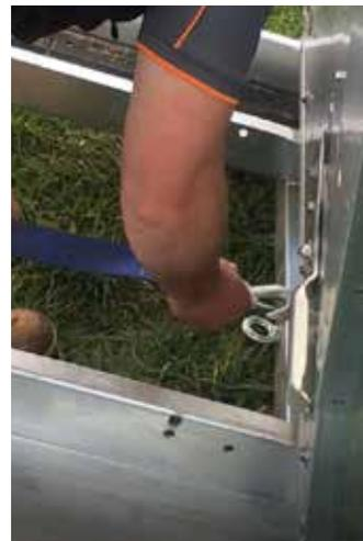
6. Unclip web strap and pull out. Thread the web strap under the centre of the feeder and connect the hook to the pull bar
