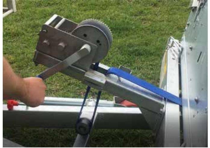
11. Winch the deck down to the trailer chassis and re-engage clutch.
