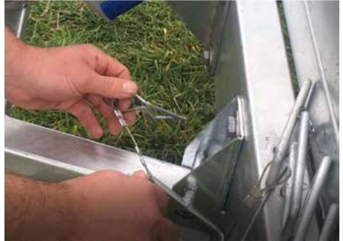
13. Apply the pivot locking pin and secure with R-clip.
