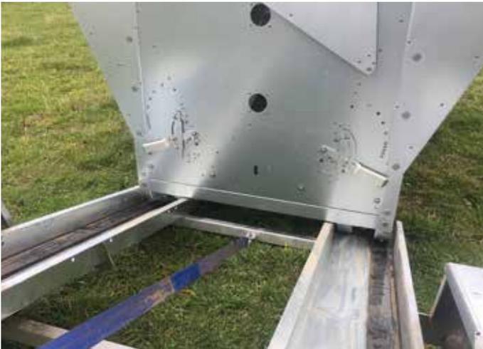
3. Continue to reverse the trailer within 50-100mm of feeder. Be sure to line up as straight as possible.
