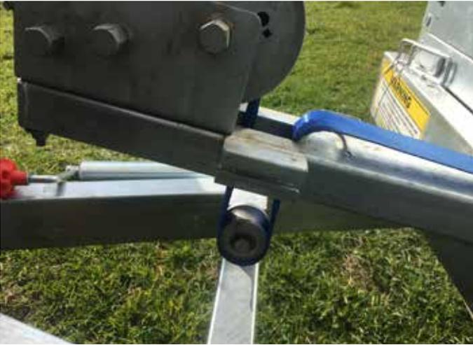
10. Disengage the winch clutch and thread the flat, untwisted web strap down and around the pulley.
