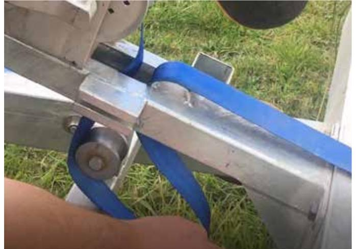
4. Loosen the web strap enough to remove it from the pulley.
