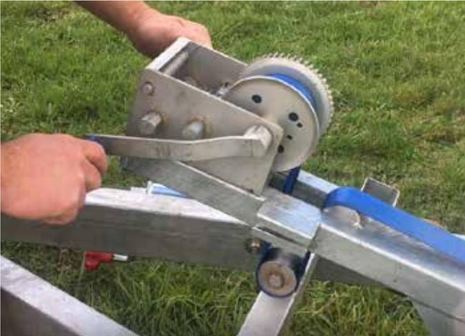
3. Release the winch clutch and leave disengaged.
