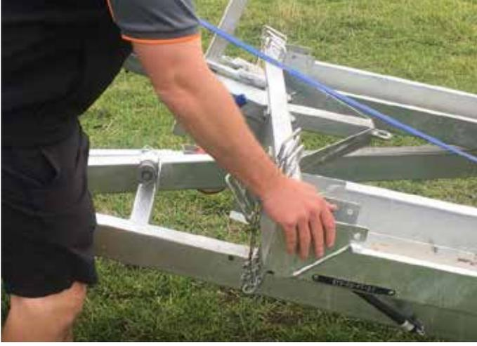
9. Lower (push down) the deck back down to the trailer chassis.
