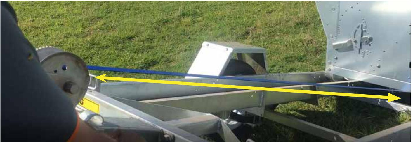
**WARNING!** Carefully guide the web strap onto the spindle. Keep the web strap flat. Ensure the web strap does **NOT** twist at any time. Ensure the web strap does **NOT** fold over whilst winching.
